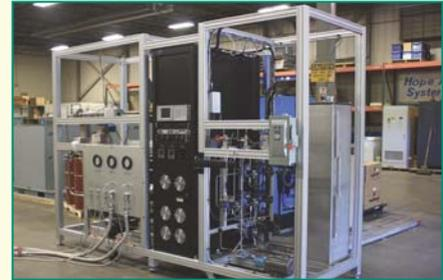
*A major manufacturer had a requirement for an integrated control system that required the design and assembly of a structural aluminum machine frame, pneumatic and automation assemblies, hose and stainless steel fittings and a PLC driven control system.*
