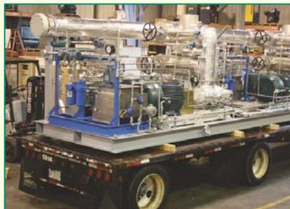
*The compact design of the skid accommodated three pump/motor combinations working in parallel, each pump drawing oil from a common supply and discharge header, and each pump/motor has its own electrical controls and protective devices.*
