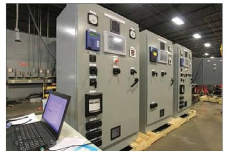
*The refurbishment included new PLC based unit control systems, one per generator, which were programmed and tested at the Sorensen Systems fabrication facility.*
