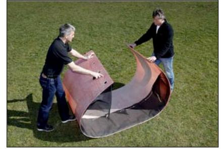
(3) Each sheet is formed into a cylinder.
