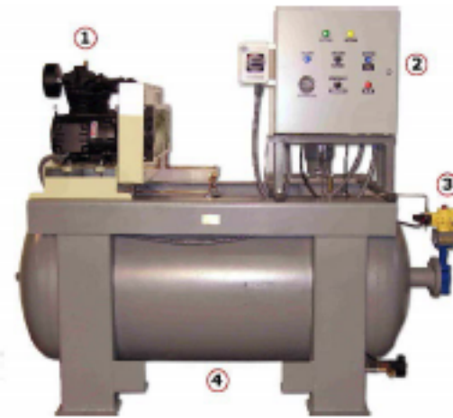
Standard components of a turn-key Airburst system: 1) Air compressor, 2) Control panel, 3) Valves and 4) Receiver.
