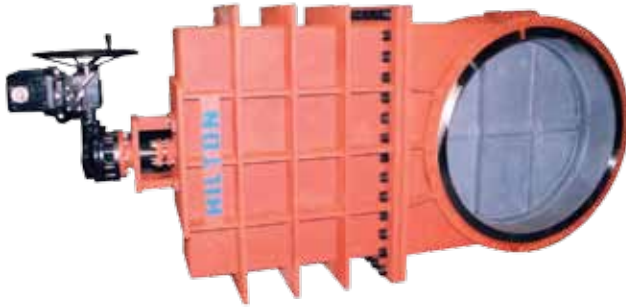
48" Wedge Gate Carbon Steel Body, Monel Trim, Belzona Interior Coating, Narrow F to F, Shipboard Seawater Cooling
