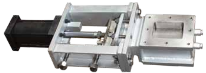
Bonnetless Knife Gate, 150 psi, 304L SS, Extended F-to-F, Purge Ports, Pneumatic, Co-Gen Plant Wood Chip Processing
