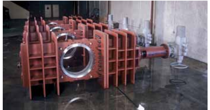
40" Thru-Port Knife Gates, ANSI 300, Removable Port Liners, Tungsten Carbide Hardfacing & Abrasion Resistant 410 SS Gate, Abrasive Mine Tailings, Kennecott Copper, Utah
