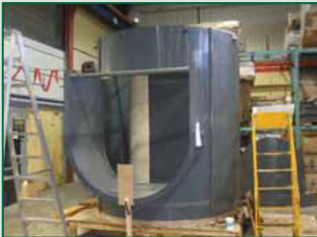
Fabrication of a 60 MGD Vortex unit Austin, Texas.
