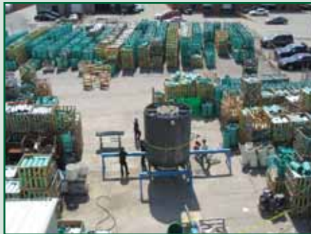
Hydrostatic testing of a large Vortex unit.
